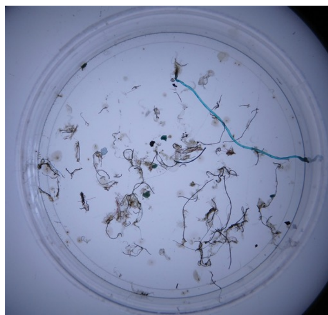
Fig. 1. Microplastics under a microscope showing all types such as fibers, pellets, and filaments (films).
