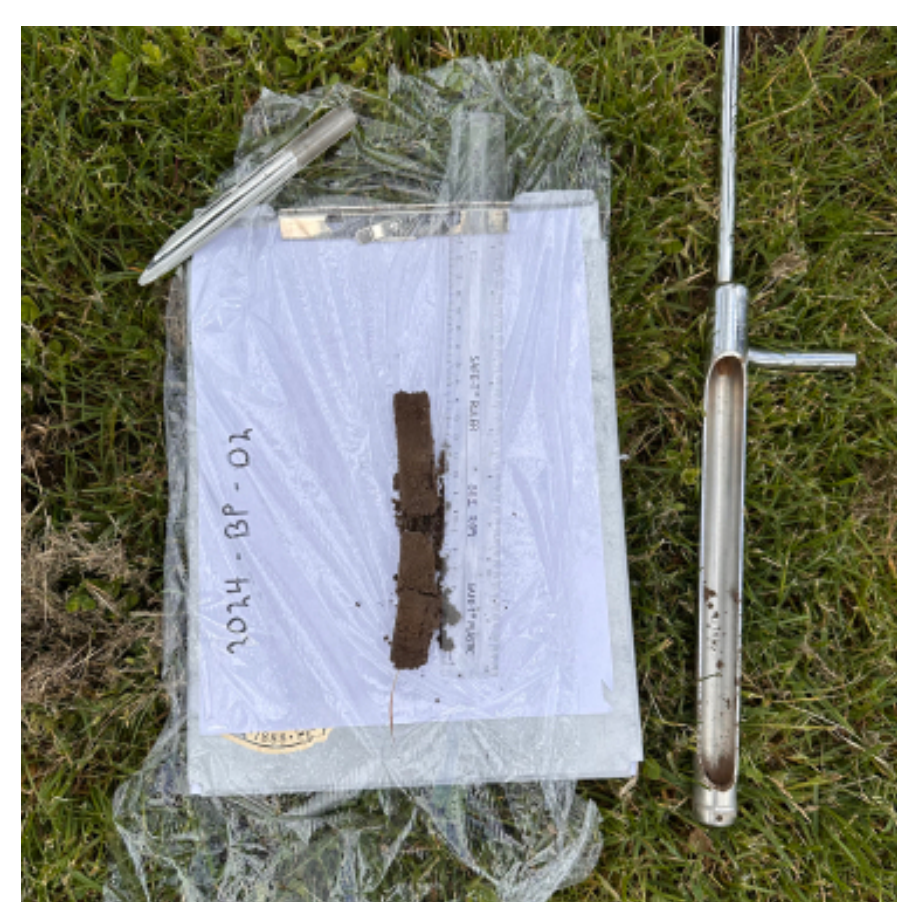
Fig 2. Cores were collected, using soil corers, from the Puyallup, Kapowsin, and Buckley associations.
