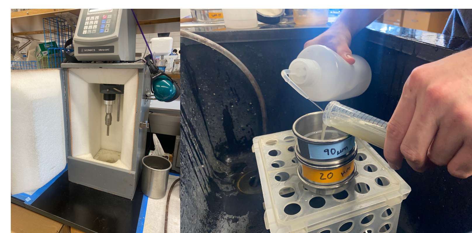
Right: Sieving of sediment samples. Left: Sonicator setup used for sediment samples.
