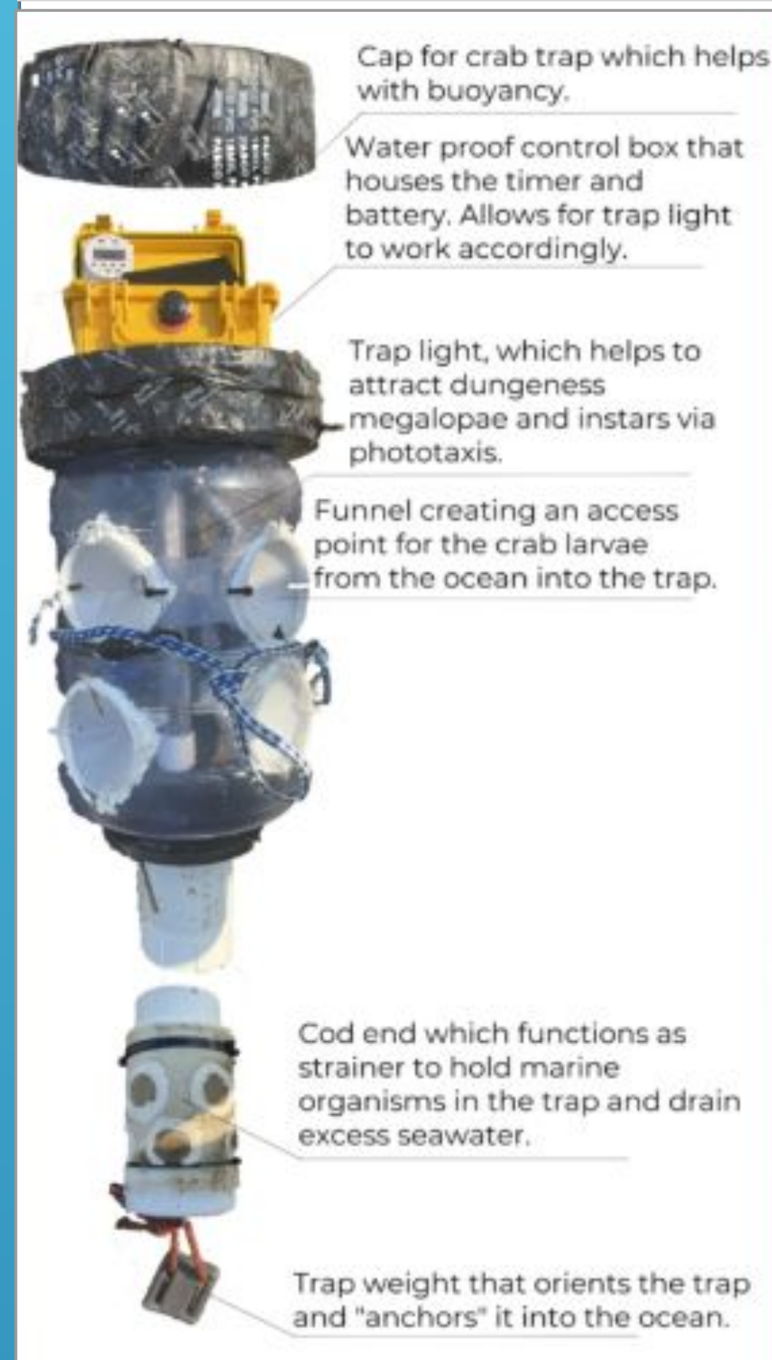
Figure 5. Diagram of the larval light trap made by UW Tacoma Lab member Prasis Pandey.
