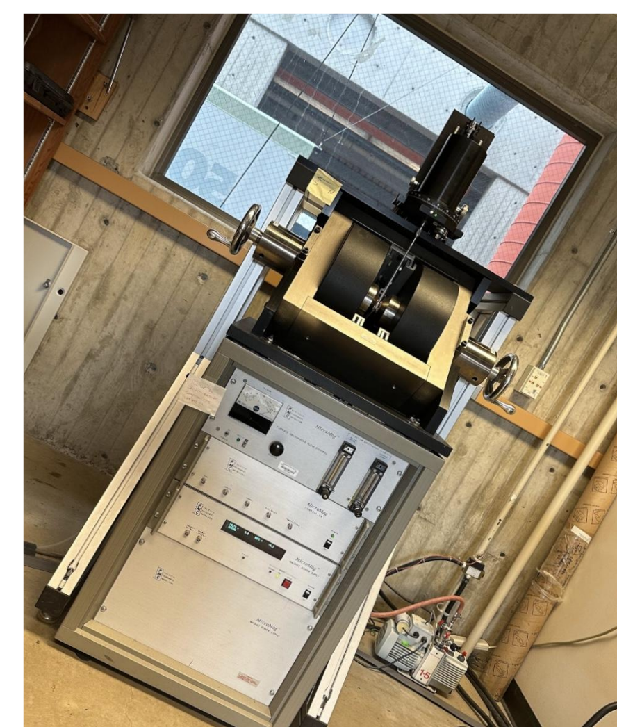
Pic 3. Princeton Measurements Corporation Micromag 3900 Vibrating Sample Magnetometer used to get IRM and hysteresis data.
