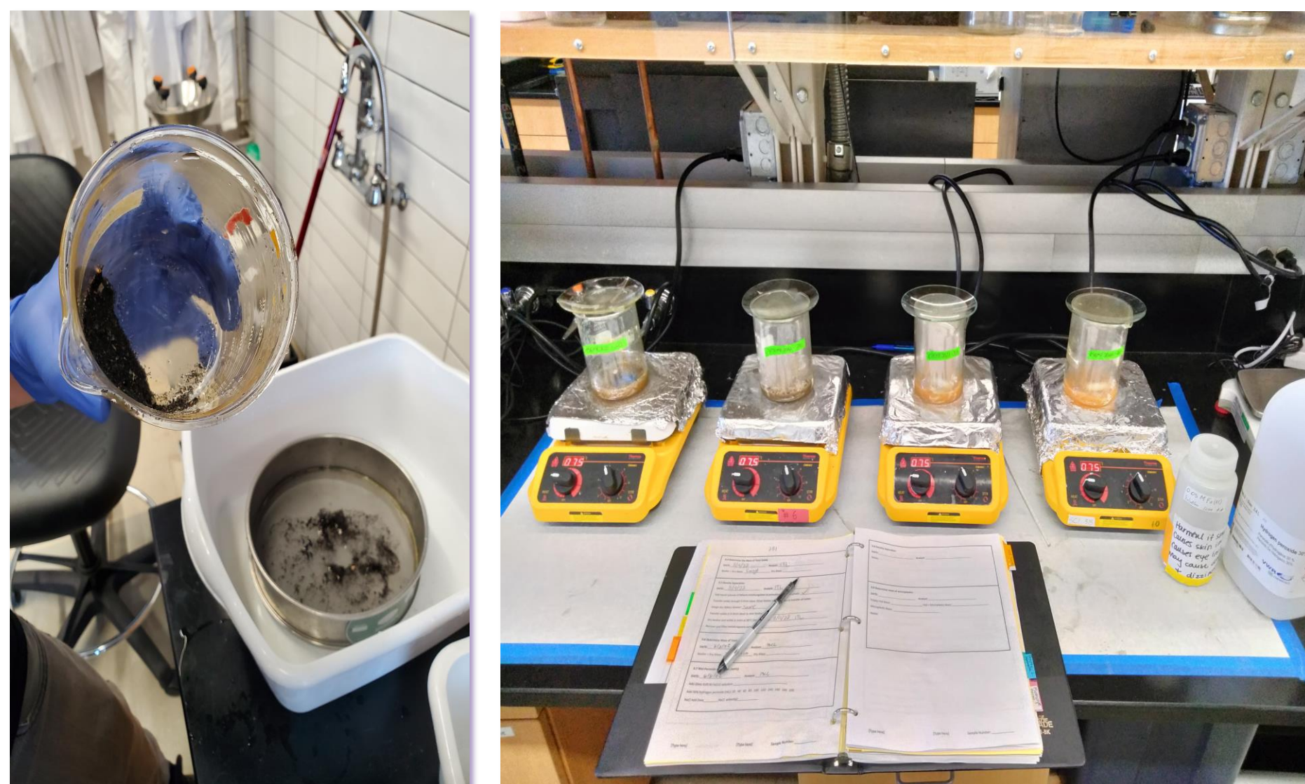
Solids left over after LMT separation and floating solids transferred to the sieve Wet peroxide oxidation
