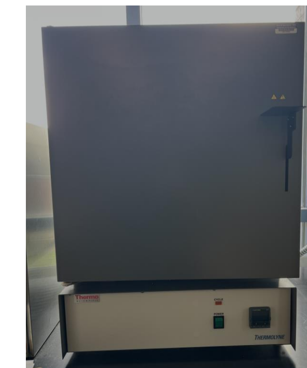
Thermolyne oven used to burn off carbon
