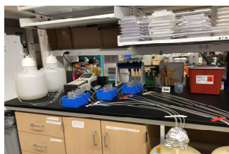
Figure 2. Tube reactor system. The tube reactor system is an apparatus used to study biofilms. A source of nutrients is continually pumped through several lines of tubing where it is emptied into waste carboys. Bacteria are injected into the tubing and allowed to grow over several days until they are ready to be harvested.
