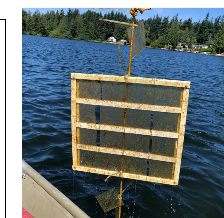
Frames and acrylic plates used to collect periphyton from local lakes/ Photo courtesy of the Gawel Lab, UWT.
