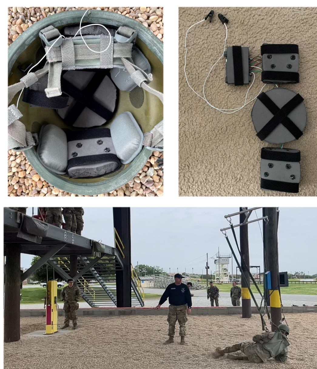
Figure 1 (top left): EEG device in helmet; Figure 2 (top right): EEG device stand-alone; Figure 3: (bottom): Ft. Benning Drop Tests. Pictures courtesy of John Tarasidis
