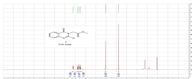
Figure 5. H-NMR data of the successful synthesis of the N-alkylation of Chloro-quinazolinone by affording methyl-2-bromoacetate in good yield 71%
