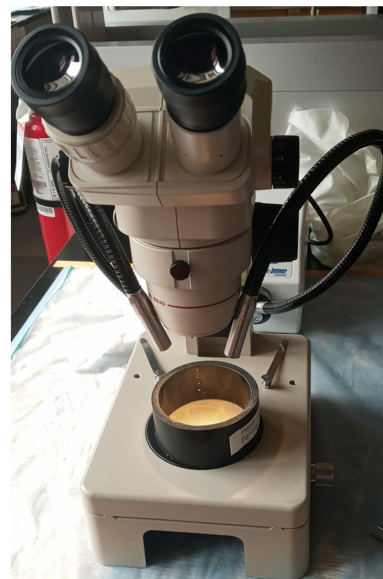
Figure 4: Microscope set up for analysis for microplastic picking Photo credit: Sade Duplis
