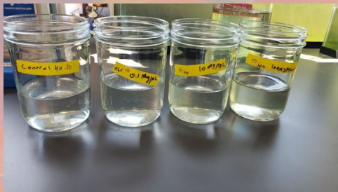
Figure 2: Serial dilution of sodium perchlorate with ADA&M, an artificial fresh water for the culture of zooplankton. Actual concentrations used after refinements of protocol are: 0, 10, & 100 mg/L of sodium perchlorate.
