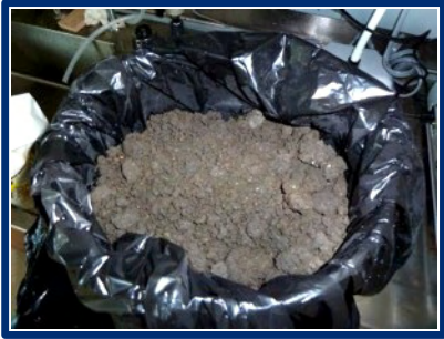
100% Class A Biosolids: carbon source nutrient source
