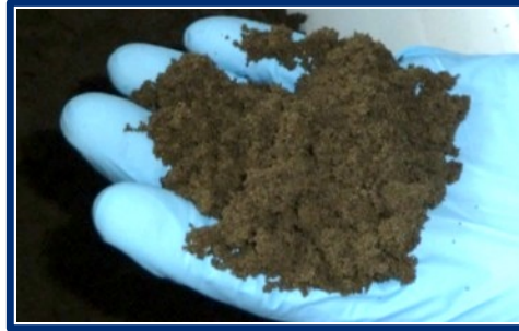
WTR (water treatment residual): aluminum and iron based capture phosphates
