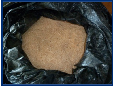
Sawdust: moisture retention carbon source
