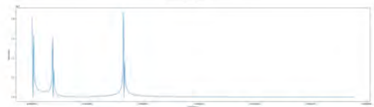
Fig. 3: Frequency domain of the synthetic data with the three highest amplitude sinusoids removed
